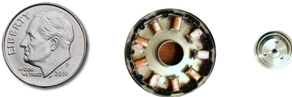
Figure 3.3 Actual generator armature and rotor next to a dime for size comparison.
