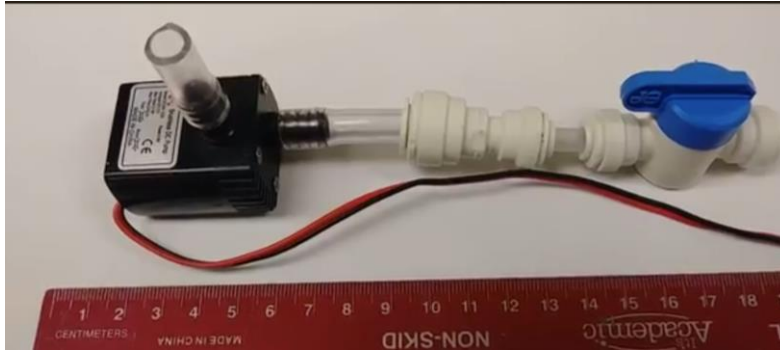
Figure 8.12 Water pump, tubing, push –fit connectors and valves used on closed-loop circuit
