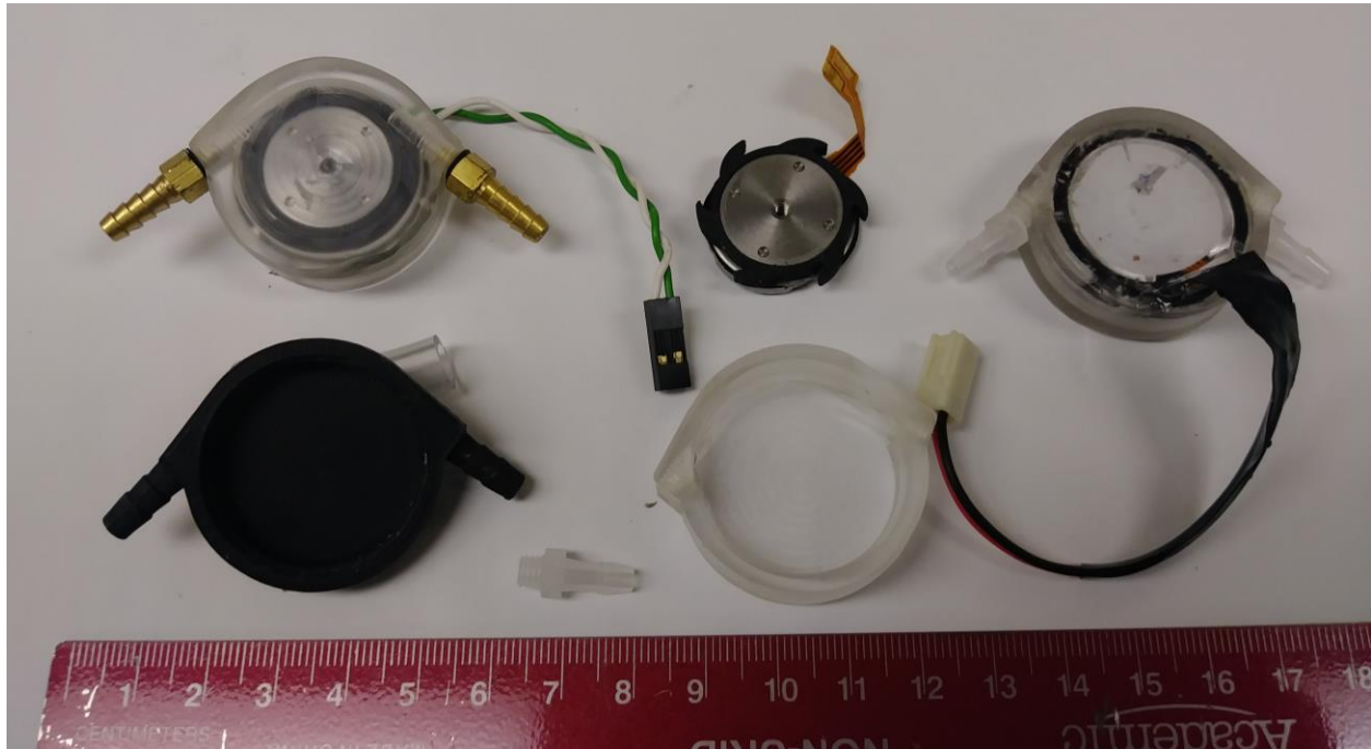
Figure 7.9 Optimized turbine for implantation (OTI-1) 3D-printed in ABS and machined in PMMA with different barbed connectors and blade-assembly-loaded generator.
