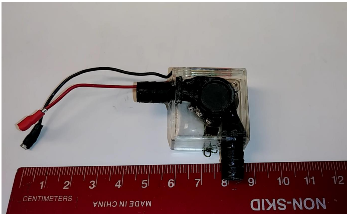
Figure 7.7 Miniaturized-scale turbine (MST) 3D printed in ABS and assembled for testing in a transparent holder.
